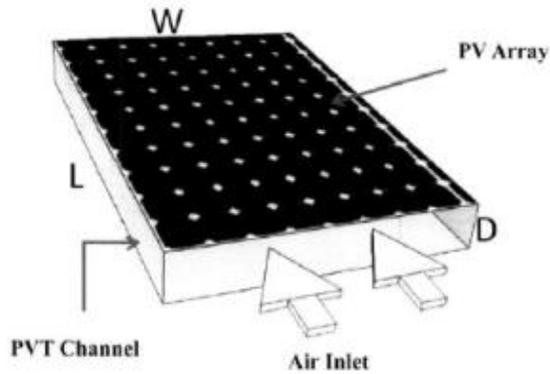
**Figure 1: A typical PVT-Air collector**
