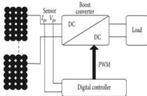
Figure 1 Block Diagram of PV Generation System
