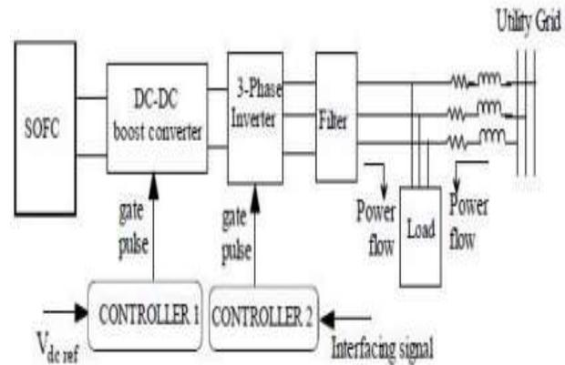
Figure 4. Schematic diagram of grid connected DGs
