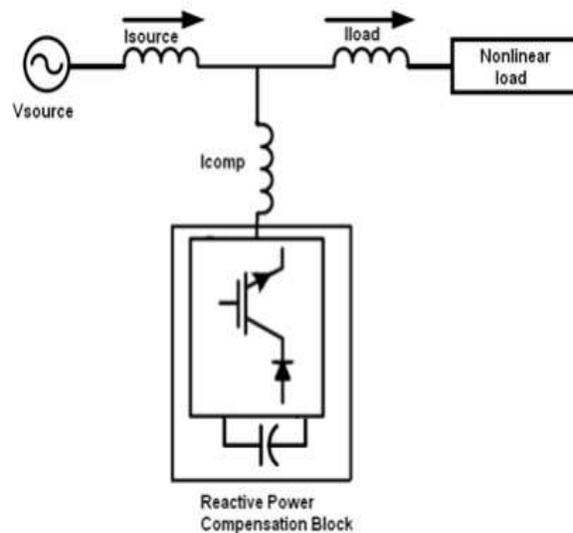
Figure 2 Parallel (shunt) connection
