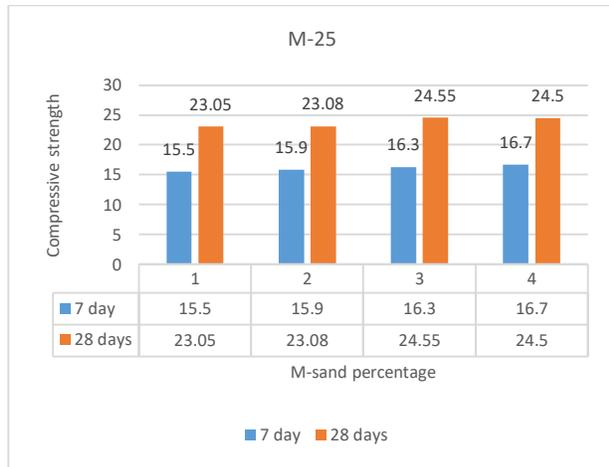
Fig. 5. Compressive Strength of M-25 mix
