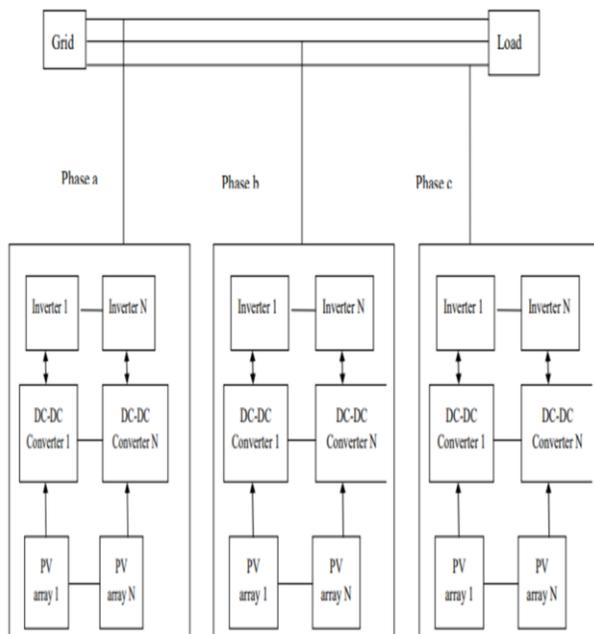
Figure 3 Block diagram of Grid-connected PV system The PV system shown in Fig.3 includes n cascaded
