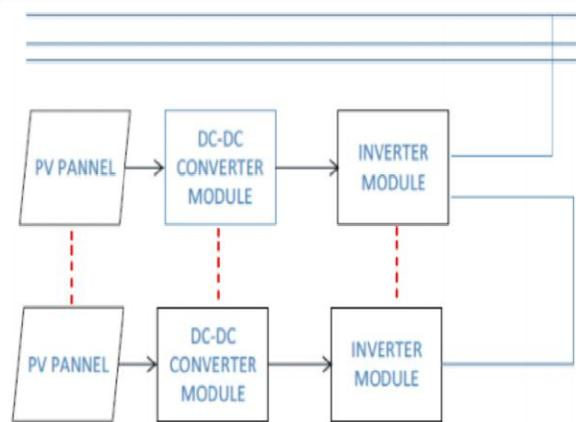
Figure 2 Block Diagram of Cascaded PV system for one phase
