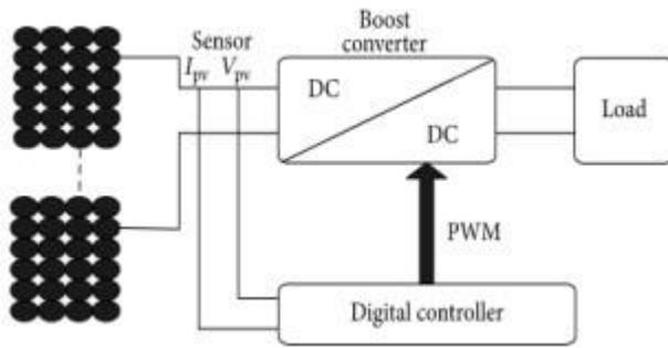
Figure1 Block Diagram of PV Generation System
