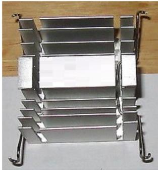
**Figure 2: North and south bridge heat sink**
