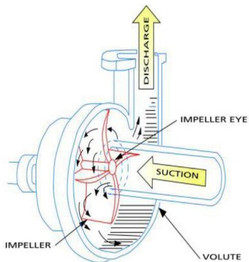
**Fig.1. working principle of centrifugal pump**
