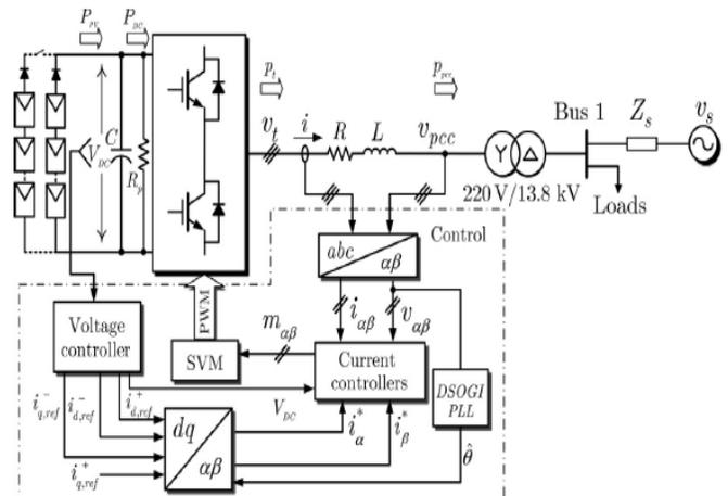
**Fig. 6: Schematic diagram of a grid-connected PV system with DC side model**
