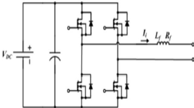
**Fig. 2: An example of power conversion unit in DPGS.**
