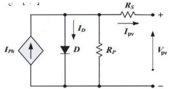
**Figure 3: Electrical equivalent circuit of PV cell.**
