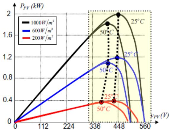
**Fig. 5 Used PV array power characteristic curves**
