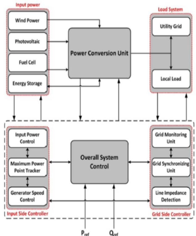
**Fig. 1: General structure of DPGS with different power sources**
