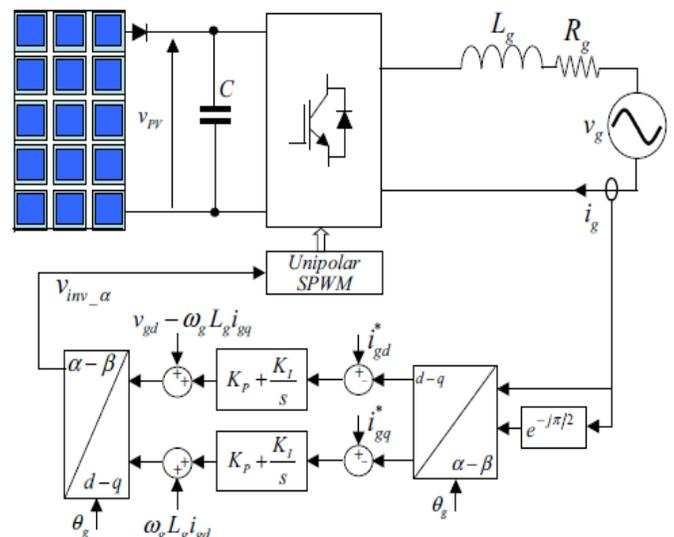
**Fig. 4: Control structure of the single-phase grid-tied inverter.**
