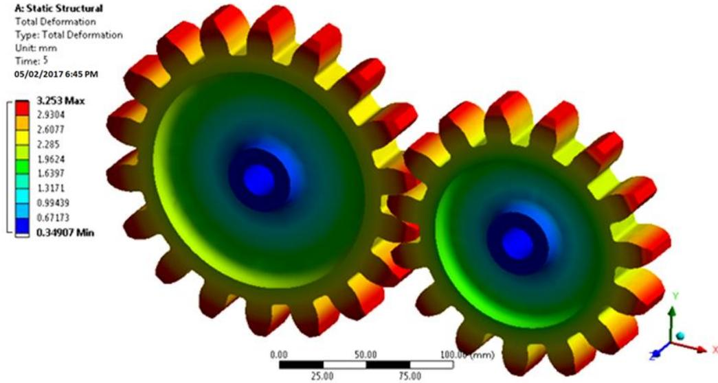
**Figure 4.5:** Total Deformation of Spur gears
