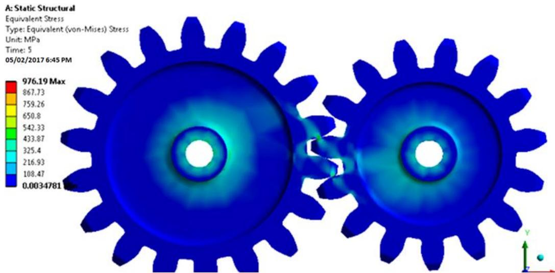
**Figure 4.5:** Von-Mises Stress of Spur gears
