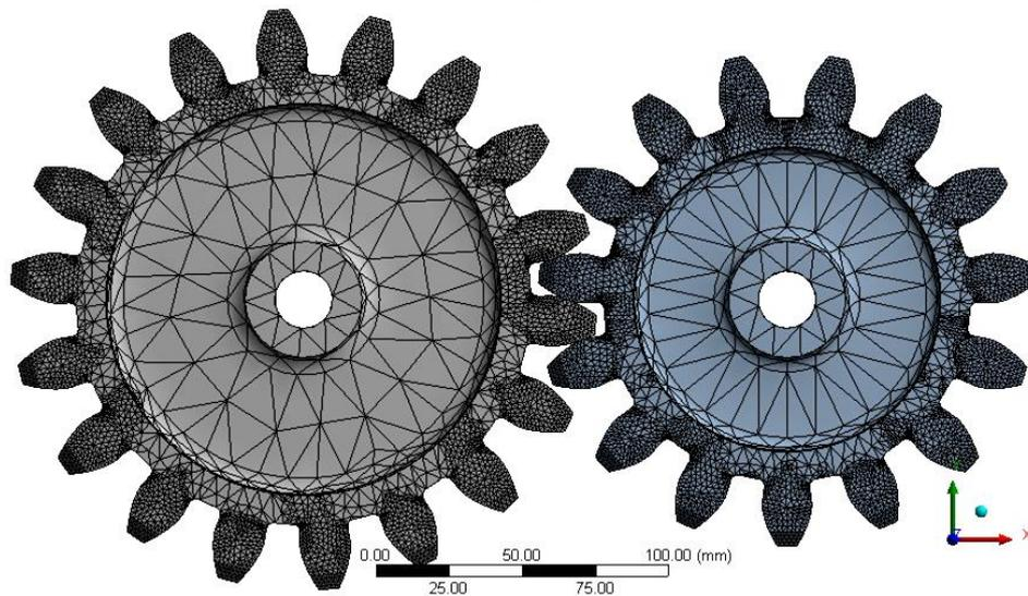
**Figure 3:** Meshed model of spur gear
