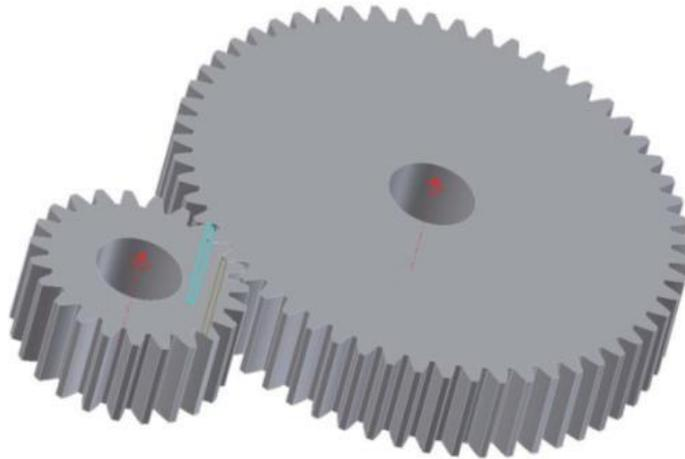
**Figure 1:** Spur gear
