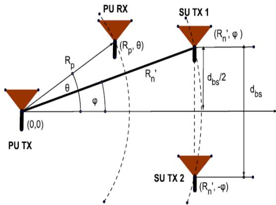
Figure 1: cognitive radio system with coordinated multipoint JT
