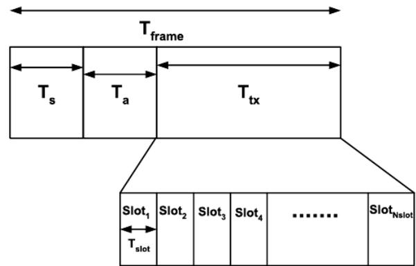
Figure 2: Distribution of time in each time frame  $T_{frame}$
