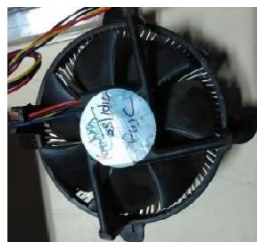
Figure 5: Complete assembly of CPU Heat sink with Fan
