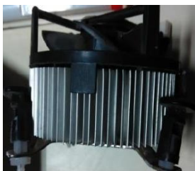
Figure 5: Complete assembly of CPU Heat sink with Fan
