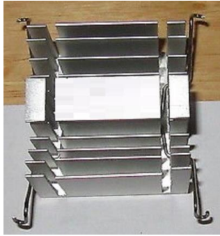
Figure 2: North and south bridge heat sink
