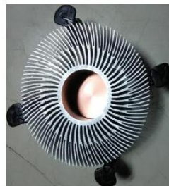
Figure 4: CPU heat sink with copper block on fan side of the motherboard
