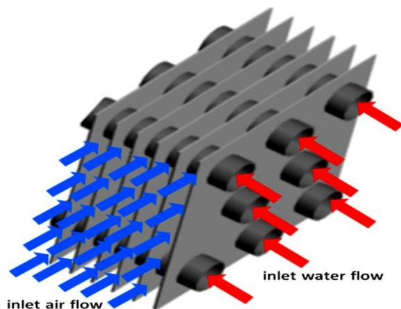
**Fig 3 design of fin plate inlet air flow**
