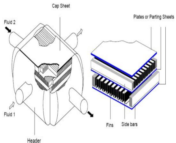
**Fig 4: Plate fin heat exchanger assembly and details Side bars Plates or Parting Sheets Fins Fluid 1 Fluid 2 Cap Sheet Header**
