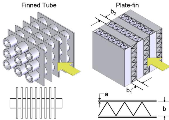
**Fig. 2 design of fin plate heat exchanger**
