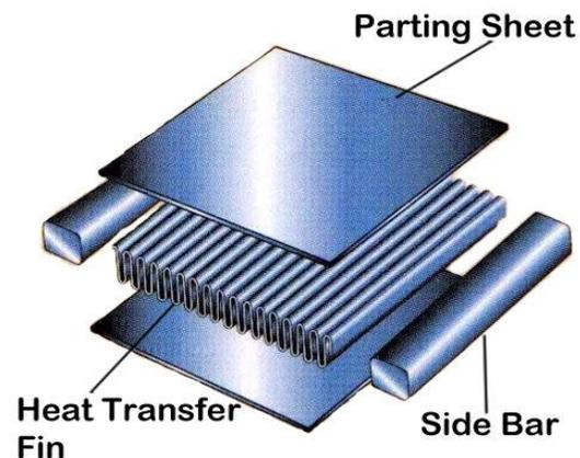
**Fig. 1 Plate fin heat exchanger**
