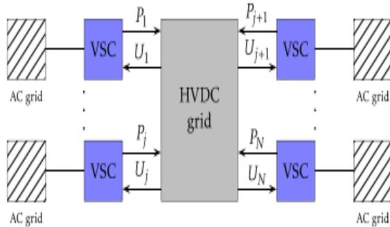
**Fig. 2. Representation of a generic MT-HVDC network.**
