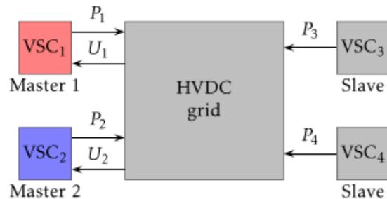
**Fig. 4. Example of a voltage margin control strategy**
