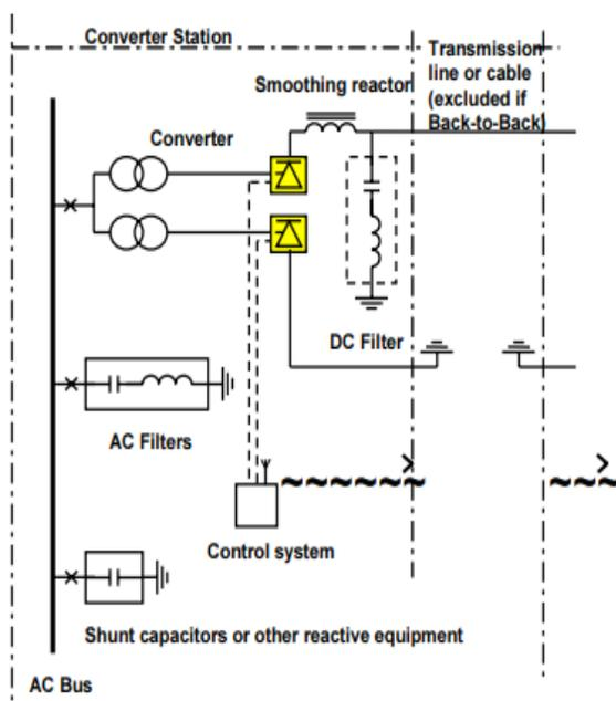
**Fig 1: components in HVDC system**
