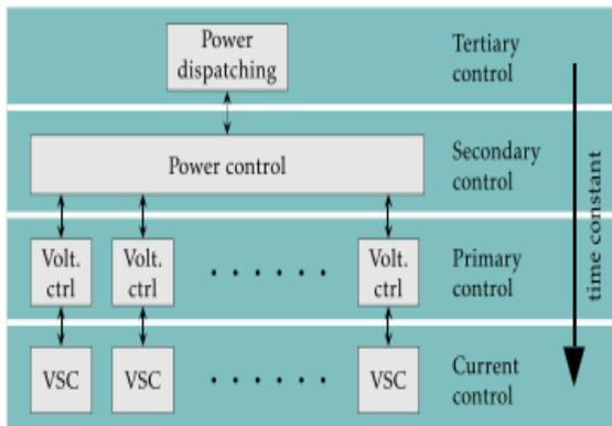
**Fig. 3. Hierarchical control structure for MT-HVDC networks.**
